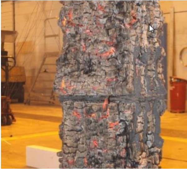
Figure 5: Fire test of glulam at SP Firetech. Standard ISO fire for 90 minutes and observation in the cooling process. This specimen has an internal steel connection
