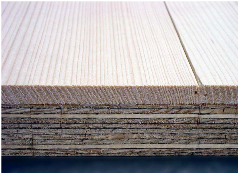
Figure 6: Radially sawn spruce laths glued to Kerto-Q panels
