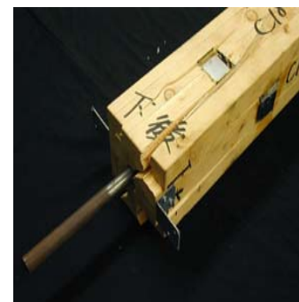
Fracture of joint
