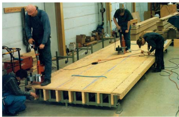
Figure 3. Screwing of the Stadler IG 6x100 mm with the spacing of 200 mm.
