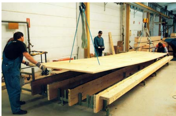
Figure 2. Assembling of the 39 mm thick Kerto-LVL skin panel with cross veneers on the 51x360 mm Kerto-LVL beams with glue spread on the edges.
