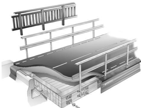
Figure 12: Illustration prestressed timber deck
