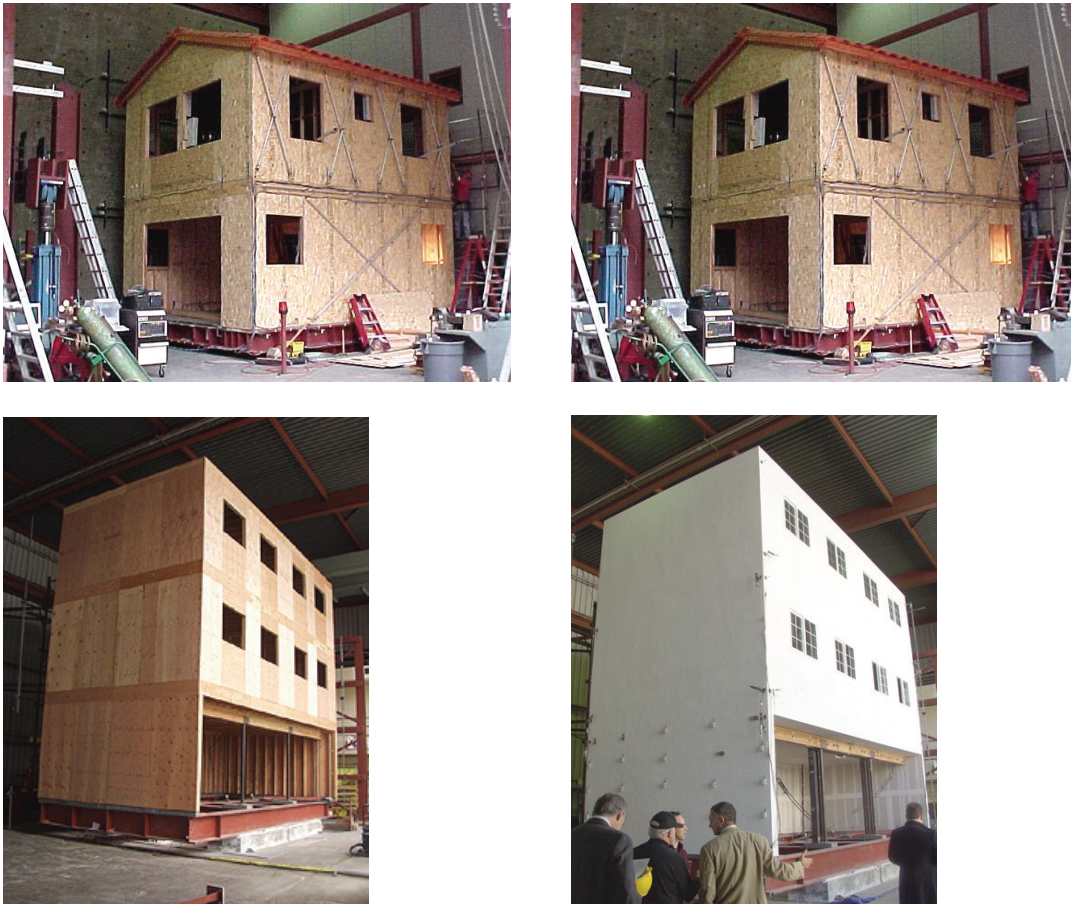
Figure 4: Shake table test structures of the CUREE-Caltech Woodframe Project (after Fischer et al. 2000 and Mosalam et al. 2002).
