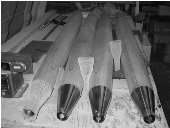
Figure 8: Stainless steel caps were used to cover the ends of the struts.
