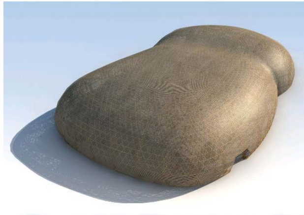
Illustration 15: (3) Finally, Bamboo Mesh (functioned as trellis, also knitted into the same hexagonal pattern) covering makes biomorphic surface shape
