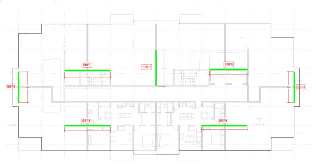
Figure 13: Floor Plan with Brace Locations
