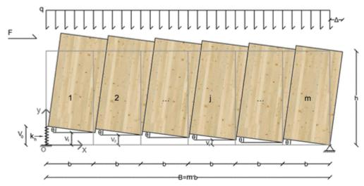
Figure 2: CLT Shear wall Deformation
