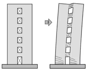
Figure 4: Concrete Shear Walls Deformation
