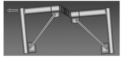
Figure 7: EBF Deformation In Canada, EBF's have no code based height limitation.
