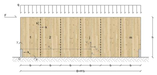
Figure 1: CLT Shear wall System<sup>1</sup>
