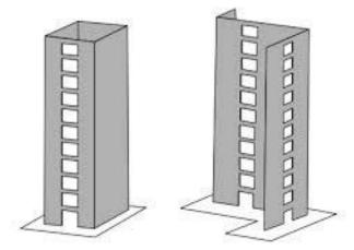
Figure 3: Concrete Shear Wall Configurations<sup>2</sup>
