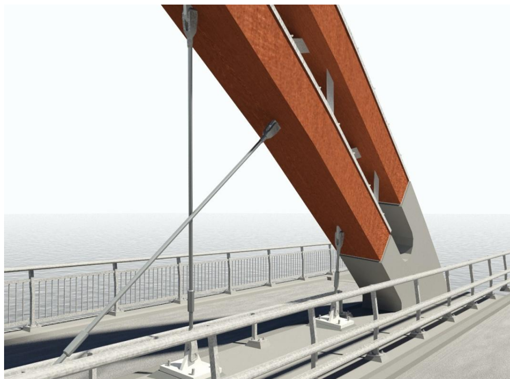
Figure 10: Detail of the hanger connections
