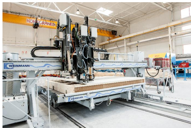
I-joists: as wall studs by the pre-fabrication of energy efficient wall panels. Photo: Ekoinbud
