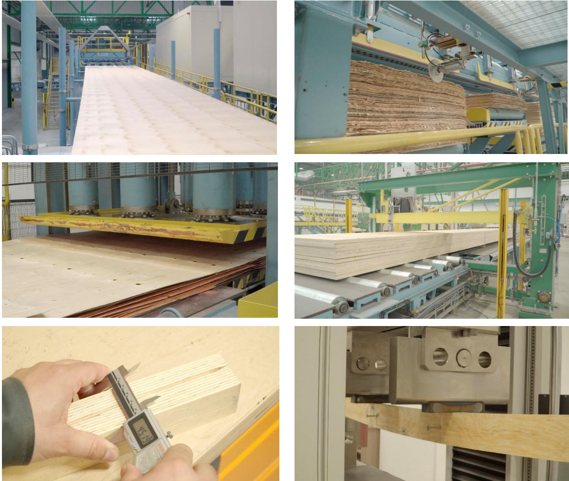
The modern production and quality control process of LVL in manufactory STEICO in Czarna Woda
