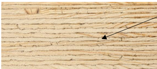
The multiple layers of 3mm laminated spruce and pine veneers. Photo: STEICO
