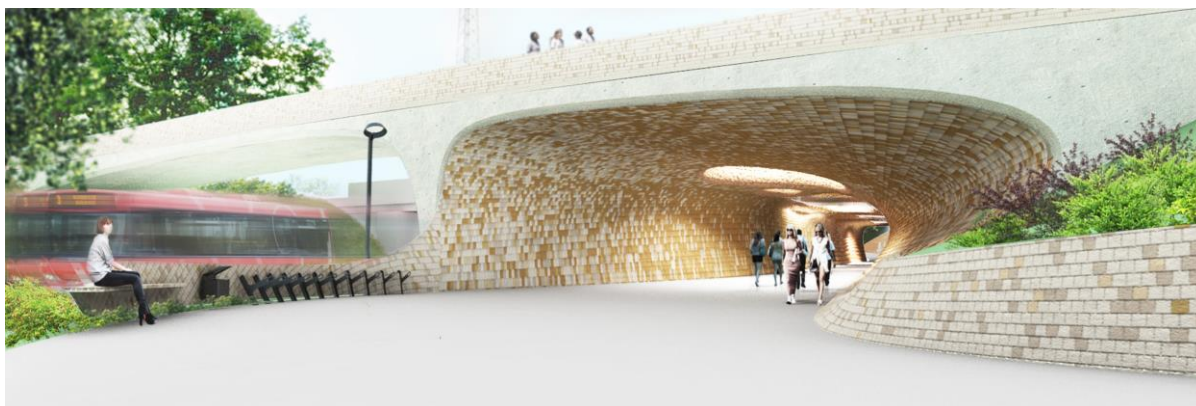
Figure 1: Tartu pedestrian tunnel and bridge competition entry. 1st prize. Freeform shingle surface, tinted according to the UV value simulations. Rendering: Practice for Architecture, Research and Theory.
