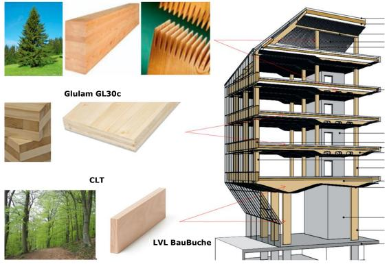
Figure 6: Different types of structural timber
