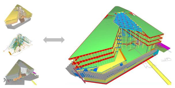
Figure 14: BIM models of different disciplines
