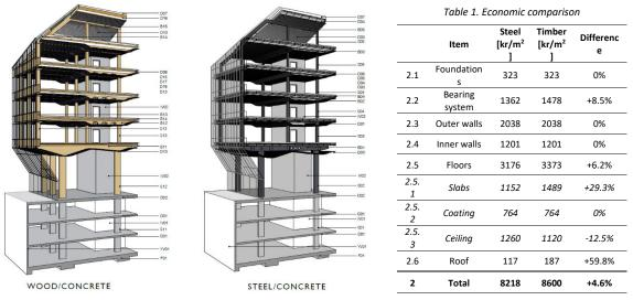
Figure 4: Study of alternatives. Cost comparison
