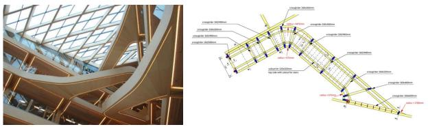
Figure 13. Main atrium stairs. Large span, helicoidal geometry, double curvature beams.
