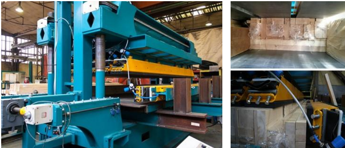
Figure 7: Large specimen production; vertical pressing over dummy elements and side pressing
