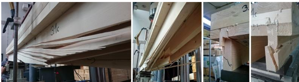
Figure 11: Damage in the XR-lam plates (either bending or shear) that occurs in several steps
