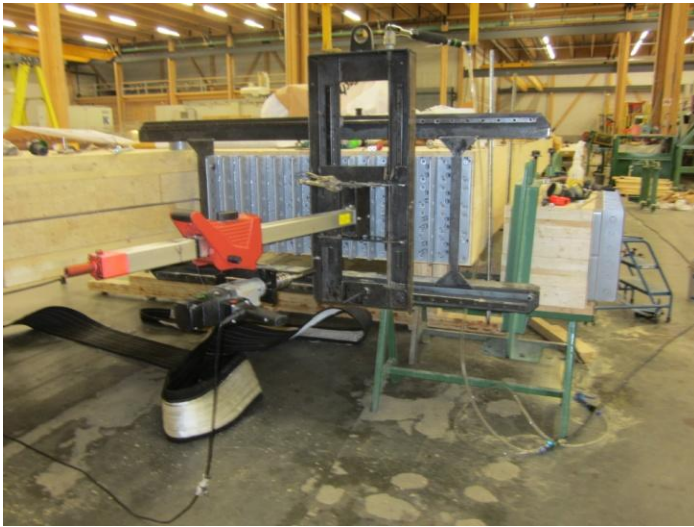
Figure 18: Setup for the installation of the transportation joint screws.
