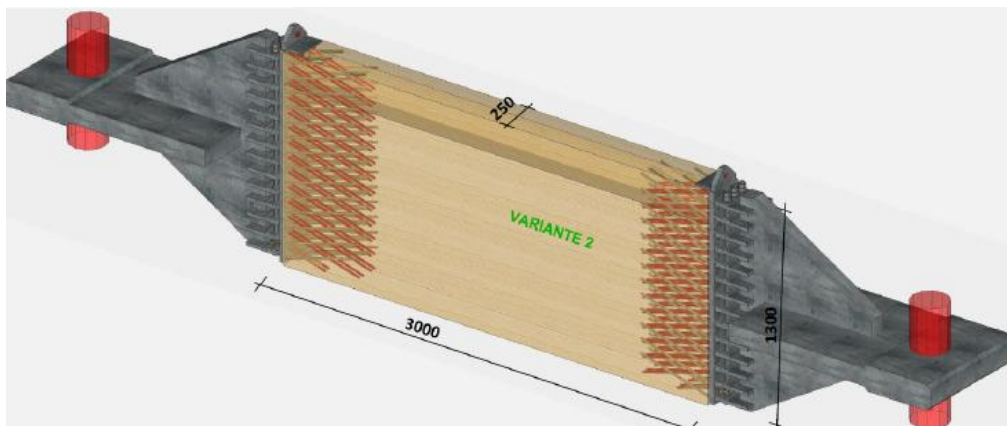
Figure 10: Test setup for the tension connection
