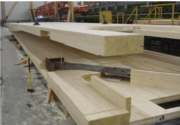
Figure 17: Fabrication of a principal beam, gluing half-parts together
