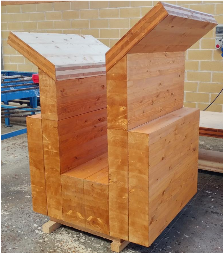
Figure 10: Mock-up of a main horizontal beam (half of the upper side with roof) aimed at studying the gutter channel and the waterproofing covering
