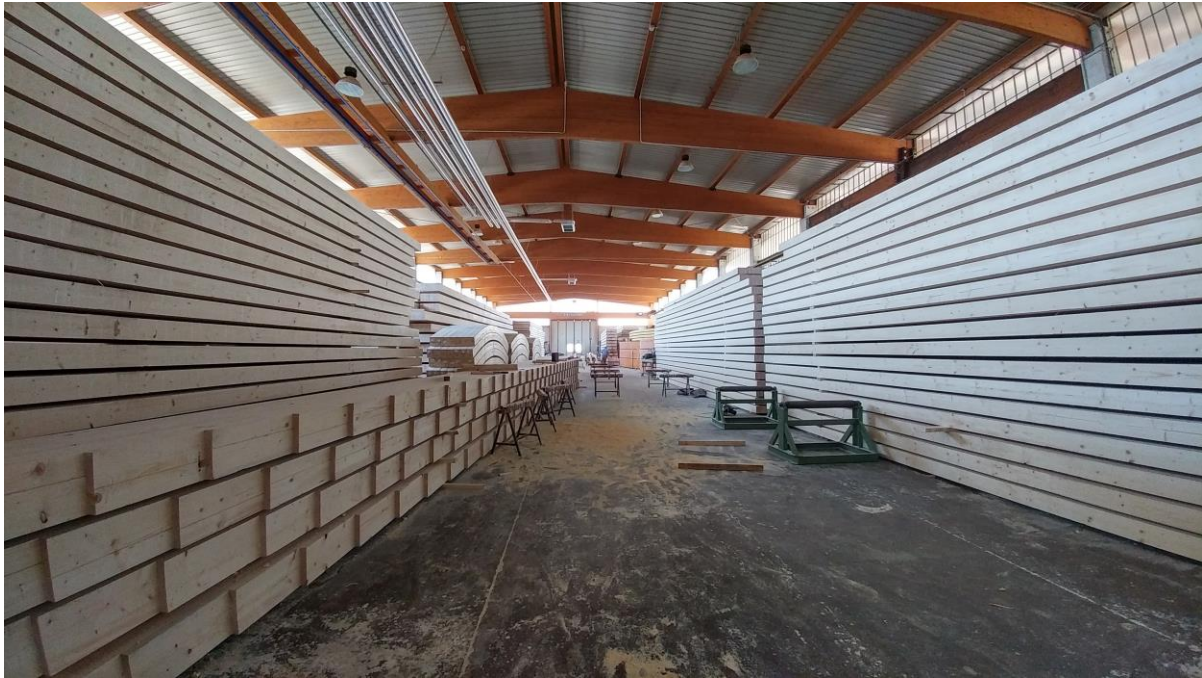
Figure 12: Factory of Rubner Holzbau Sud a Calitri (AV) Italy, glulam beams ready to be pre-assembled
