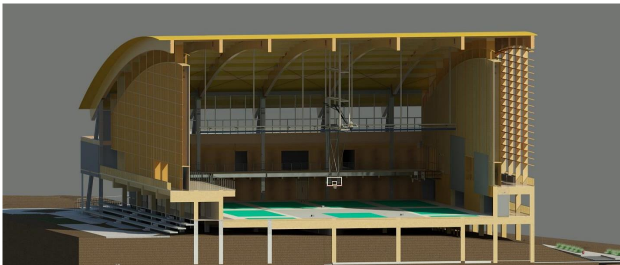
Figure 3: cross section view of the sports hall
