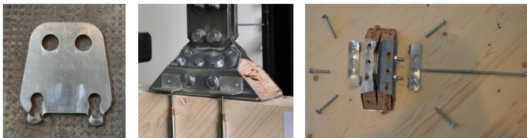
Figure 13: Failure mode in tension configuration (left) and shear configuration (right)
