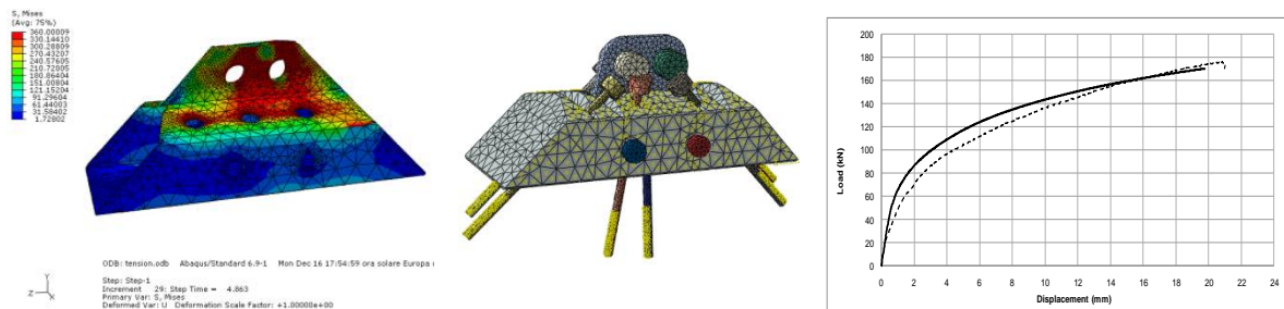
Figure 16: View of FEM Abaqus models (left) and comparison between the load – displacement curve obtained by experimental test -dashed line- and numerical mode -continuous line- (right)
