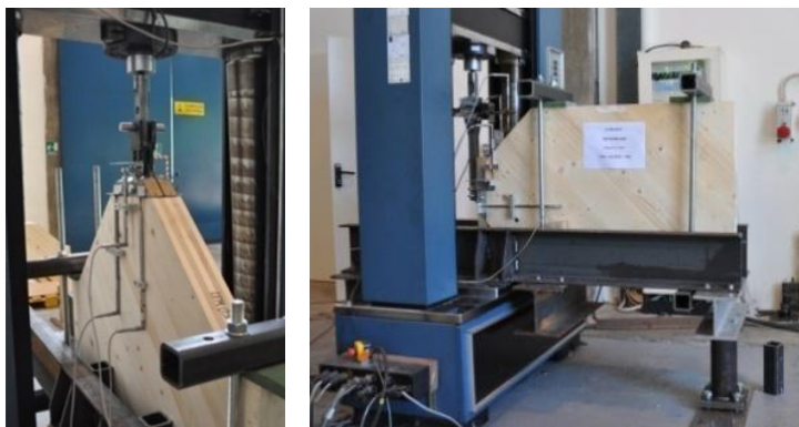
Figure 11: Setup adopted for tension configuration and shear configuration
