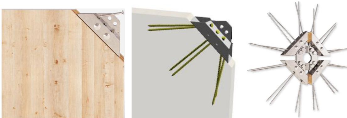
Figure 1: Schematic view of the new connection fixed at a CLT panel and a joint between 4 connectors
