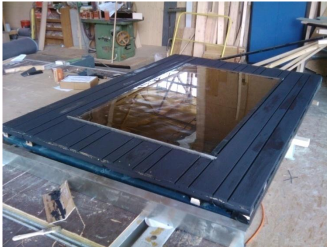
Images 11 and 12: First sample of the solar thermal collector built in a TES-Façade in the factory.
