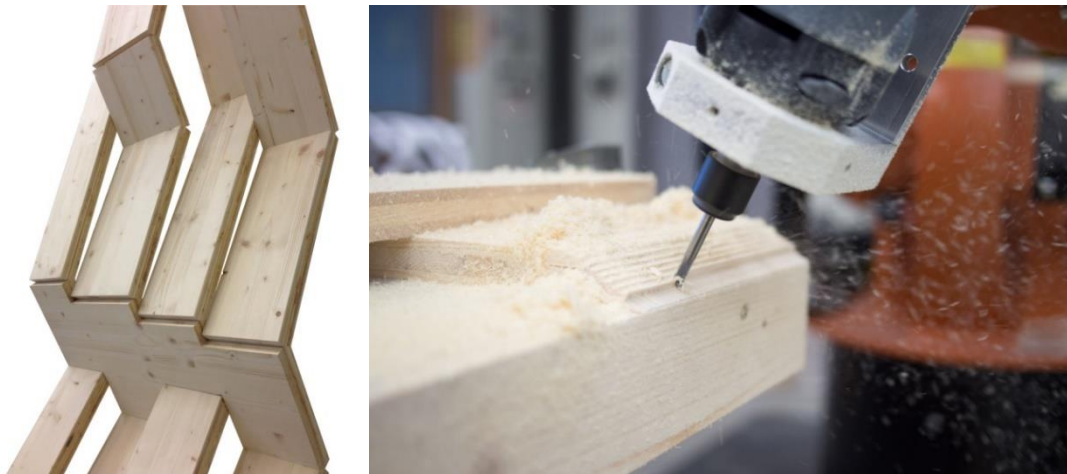
Flexible joint system with laminated plywood panels (left) and milling of angled connection parts (right).
