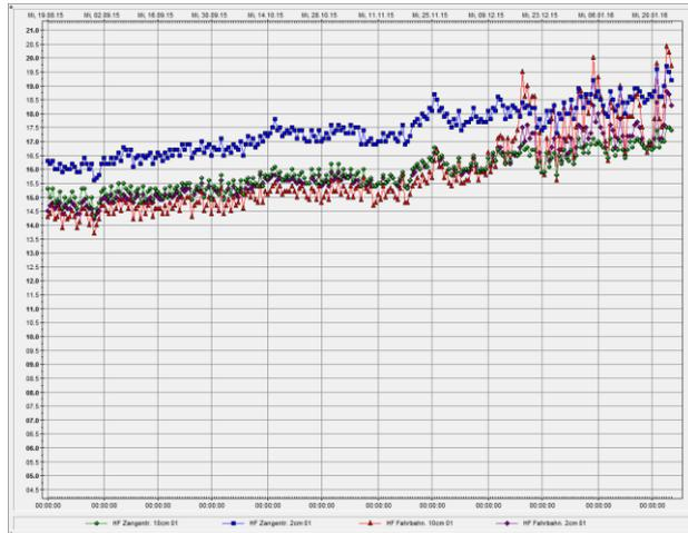
Figure 4: data output of a wood moisture recorder
