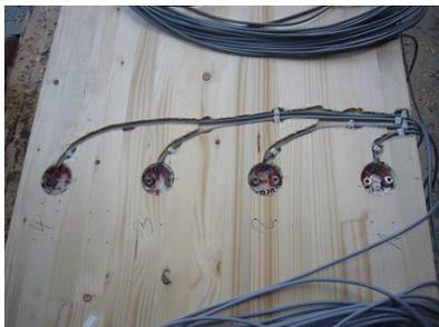
Figure 12: permanent control of wood moisture
