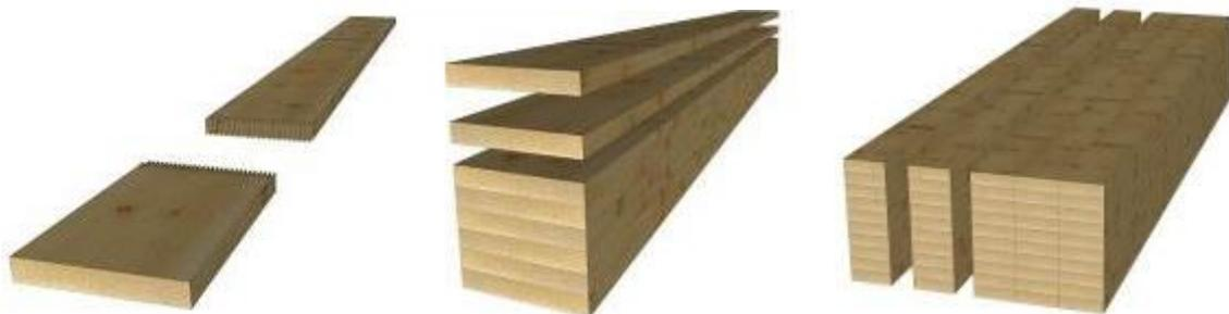
Figure 1: process of block lamination
