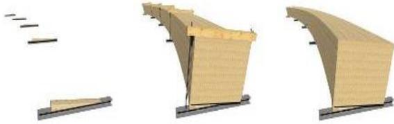
A part from curved gluing, through block lamination stepped beams are feasible both in cross section and in longitudinal section. There for glulam beams with different height or length are block-laminated to one block beam.
