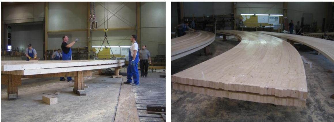
Figure 2: vertical block lamination
