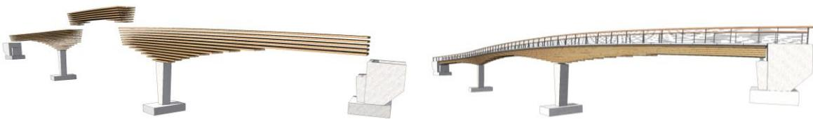
Figure 6: exploded view curved beam bridge
